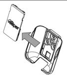
Remove the cover plate by inserting a small screwdriver into the tabs. Alternatively push the cover from the rear.
