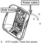
H1P cradle. Feed the power cable into the power cable hole. Use marine sealant to waterproof holes if mounting externally. Note - Side holes allow optional surface mounting.
