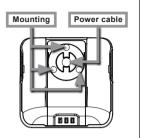
Use the cradle as a template for marking the mounting holes.
