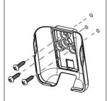
Secure with fastenings of your choice. Use marine sealant to waterproof holes if mounting externally.
