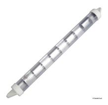
The radar reflector made of aluminium elements crossed at several 90° angles in a plastic container; very high reflecting rate, practical, highly compact. 2m² reflecting surface guaranteed up to 2, 5 nautical miles.
