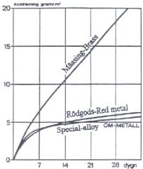
This diagram shows that the alloy used in the Isotherm skin fitting is salt water resistant and superior to red brass. The Isotherm SP skin fitting supplier was founded 1925, has ISO 9001 quality system approval and has produced more than 4 milj. skin fittings in this special alloy since they started 1974. They are suppliers to all major boatbuilders in Europe.
