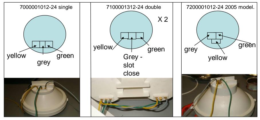
Each cable has its position and needs to respect cable colour in each slot, <u>yellow = common.</u>
