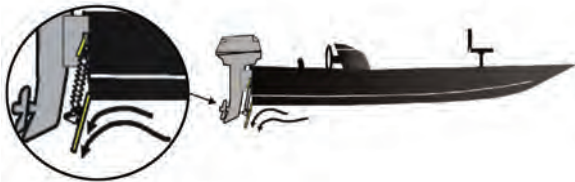
WHEN DOWN, THE PROTROLLER SMART TABS ACT AS BRAKES TO REDUCE TROLLING SPEEDS BY UP TO 35% WITHOUT LOSING STEERING CONTROL.
