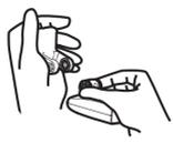
**NOTE:** The ratchets are keyed. Make sure that the square teeth on each ratchet face the square teeth on the transducer knuckle, and the triangular teeth face outward.
