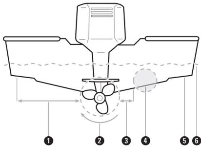
**1 Avoid areas where there is turbulent water flow.** Turbulent water is normally confined to areas immediately aft of ribs, strakes, or rivets on the bottom of the boat, and in the immediate area of the propeller(s). The best way to locate turbulence-free water is to view the transom while the boat is moving.
