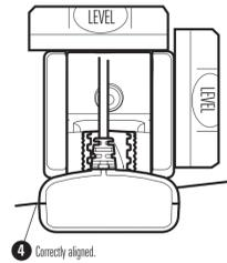
**Downward Slant:** The transducer has a natural downward slant of 4 to 5 degrees from leading edge (closest to the boat transom) to trailing edge (farthest away from the boat). Looking at the back of the transducer, the seam should be slightly below the bottom of the hull.
