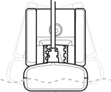
4. Once finalized, mark the correct position on the transom by tracing the silhouette of the transducer mounting bracket with a pencil or marker.
