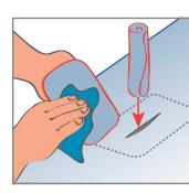
**3.** Mix half of the Polymarine adhesive & cure (3026 two part adhesive) as directed on the tin. Brush onto the surfaces thinly, the surface should look wet. Allow the adhesive to dry for at least 30 minutes.
