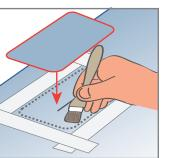
with a Smoother or Roller. Check that all the edges are stuck down. You must make sure that there is no air trapped between the surfaces. Remove the tape and rub off any excess adhesive. If the adhesive is left on it will turn brown.
