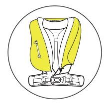
**2.** Lay the inflatable bladder on a table, as flat as possible.
