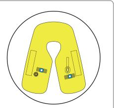
**6.** Make sure the Lume-on is well stuck on the bladder by applying finger pressure all around the sticker.
