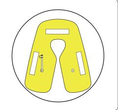
**3.** Turn the bladder over, you do NOT need to remove the bladder from lifejacket.
