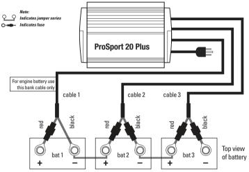
Three 12 VDC Batteries connected with a (2) series jumper for a 36 VDC Trolling Motor
