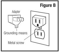
Use of an adapter is not allowed in Canada. If a grounding type receptacle is not available, do not use this appliance until the proper GFCI protected outlet is installed by a qualified electrician.
