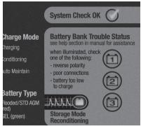
ProSport includes 7 LEDs for operation status and up to 3 battery bank trouble LEDs depending on the model.
