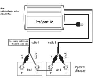
Two 12 VDC Batteries connected with a series jumper for a 24 VDC Trolling Motor
