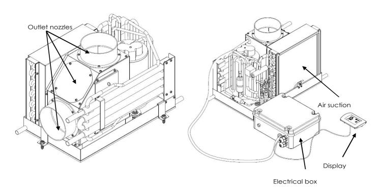
**IMPORTANT!** All nozzles can be ducted allowing the highest air flow rate, however in case of restricted space for installation, only one nozzle can be ducted while the other shall be closed.
