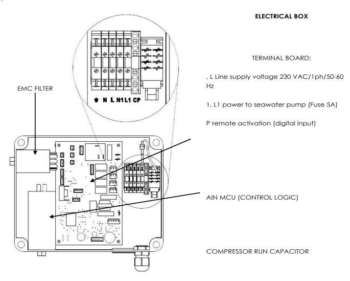
**CP**: contact for remote compressor activation, when closed the unit works normally and can be managed via thermostat display or Remote Control, when CP is open the unit goes into stand-by and cannot be activated by thermostat display or Remote Control, SB is shown on the display to indicate this condition.
