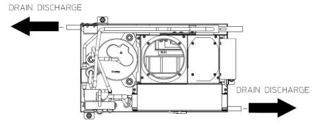
**NOTE:** The direct discharge at side is not recommended because of sucking bad smells from the outside caused by the exhaust gas of its own or other engines.
