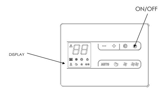
The room thermostat has to be connected with the MCU through the 6 m length cable (supplied with the unit).
