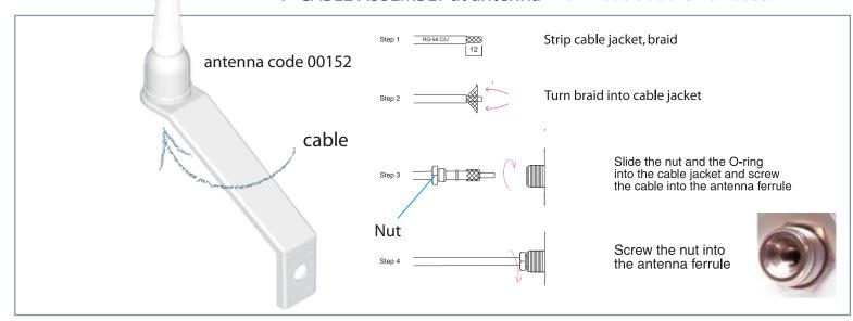
2 - Mount the antenna; for mounting the connector PL radio side, use the instruction below:
